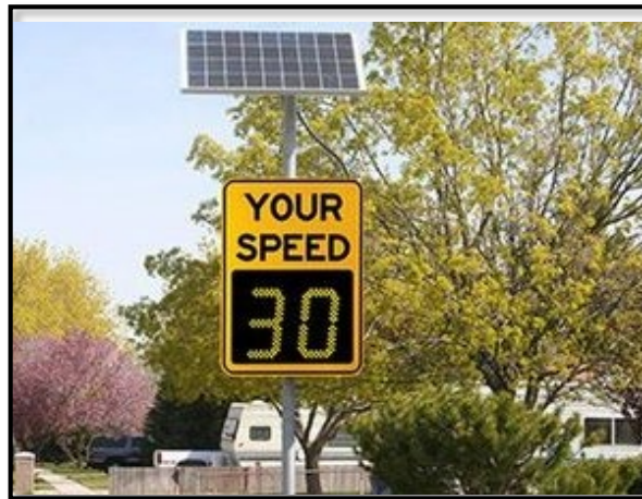
R26- Install dynamic/variable speed warning signs
