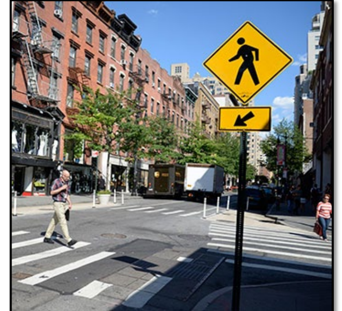
NS06- Install/upgrade larger or additional stop signs or other intersection warning/regulatory signs
