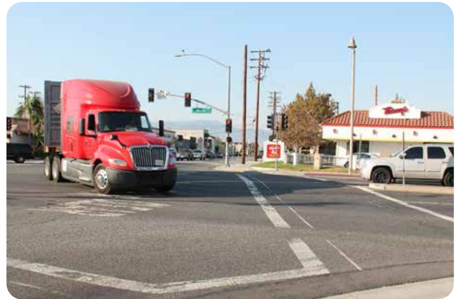
Example of 18-wheeler truck taking a wide turn onto Whittier Boulevard from Durfee Avenue, as well as other vehicles queuing at traffic signal.
