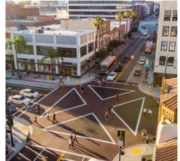
Example of scramble crosswalk in Pasadena, which could be an upgrade of the high visibility crosswalks completed during Phase 1.
