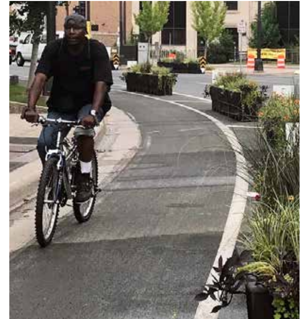
Example of painted protected bicycle lane in a pilot condition with planters as a buffer from moving vehicles.
